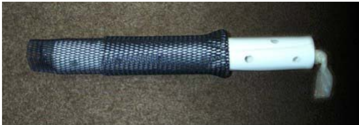
Figure 4-3. Dialysis sampler with internal PVC support shown (~ 1.25 inches in diameter by 14 inches long)
