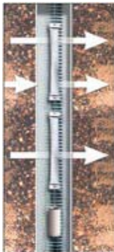
Figure 8-1. Deployment of PDB samplers to vertically profile well
