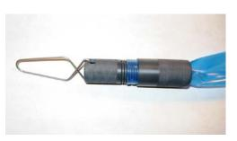
2. Insert the male threads of the top portion of the PVC Collar into the HydraSleeve. Do not insert the threads past the weld line in the HydraSleeve. NOTE some of the male threads will remain exposed, they will not be threaded entirely into the female portion.
