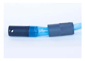
5. Insert another clip into the hole at the bottom of the HydraSleeve, under the knot. Then attach an 8-ounce bullet weight to the bottom clip.
