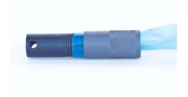
When resting on the bottom of the well, the collection cycle will begin ~54 inches off the bottom. It will fill within a 10-foot saturated screen using a single pull stroke. For screens that are less than 10-feet, the unit can be oscillated up and down to allow it to fill. The NEW 1-inch SkinnySleeve holds 300 mls.
