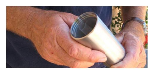
Thread stainless steel weight (or small PVC ring when using collars) (female thread) onto PVC top piece (male thread) locking the top of the HydraSleeve SS between the threads.
