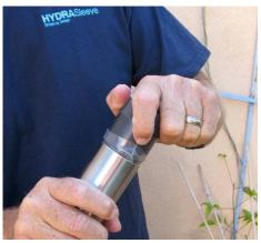
Ensure that the pieces are securely threaded together. Hold the top portion in one hand and the bottom portion in your other hand and try to pull them apart. If threaded properly they will not come apart and the SuperSleeve should be securely locked in between the threads of the 2 weight pieces.
